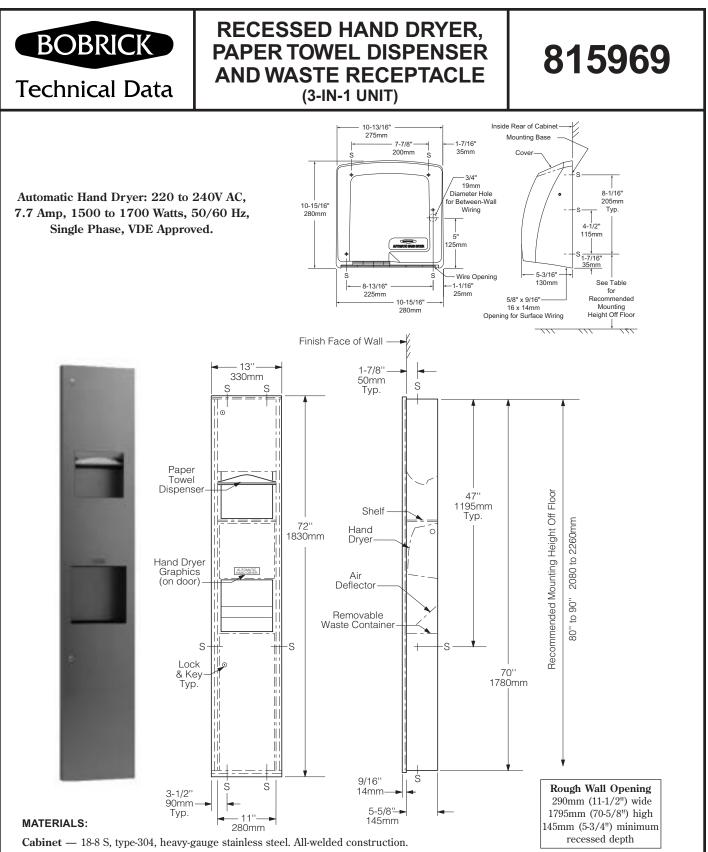
**Door** — 18-8 S, type-304, 1.2mm (18-gauge) stainless steel. 14mm (9/16")  $90^{\circ}$  return for maximum rigidity. Secured to cabinet with a concealed, full-length stainless steel piano-hinge. Equipped with a stainless steel cable door-swing limiter and two tumbler locks keyed like other Bobrick washroom accessories.
