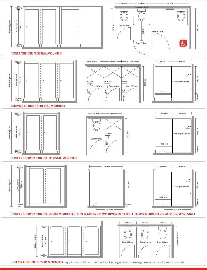
Rynat Partitioning Systems are installer friendly A full set of installation instructions including layout plans are provided. All panels are pre-drilled for ease of installation. Tool kit and all necessary fixings included with each partitioning system supplied. Full Specification and Detailed Drawings available at www.rynat.com
