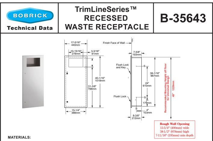
Cabinet — 18-8, Type-304, heavy-gauge stainless steel. All-welded construction. Exposed surfaces have satin-finish.
