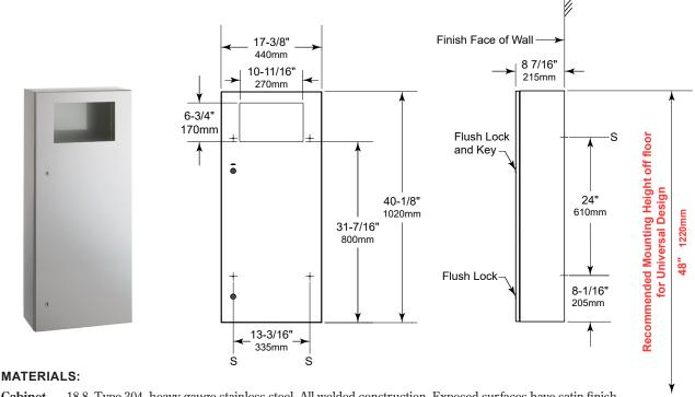
Cabinet — 18-8, Type-304, heavy-gauge stainless steel. All-welded construction. Exposed surfaces have satin-finish.
