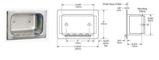
Rough Wall Opening 6" (150mm) wide 4" (102mm) high 4" (100mm) minimum recessed depth
