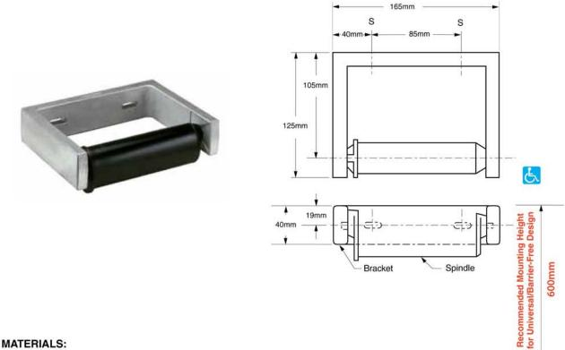
Bracket — Heavy-duty cast aluminum with satin finish. Small extrusion limits rotation of spindle to 3/4 revolution.
