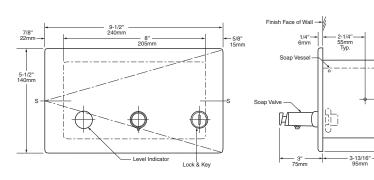
Rough Wall Opening 8-3/8" (210mm) wide 4-3/8" (110mm) high 3-7/8" (98mm) minimum recessed depth
