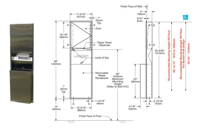
Rough Wall Opening 16" (406mm) wide 54·3/4" (1390mm) high 4" (100mm) minimum recessed depth
