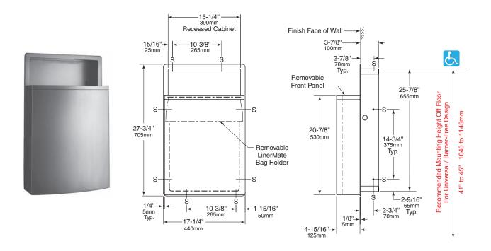
Rough Wall Opening 15-7/8" (405mm) wide 26-1/4" (665mm) high 4" (100mm) minimum recessed depth
